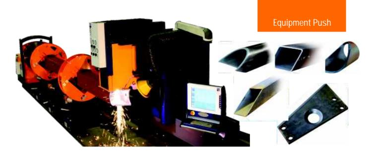
dedicated machine for profiling of pipe alone. The Multiple Profile cutter comes in several possible configurations making it a versatile multipurpose machine. These configurations allow the machine to cut pipes, box sections (SHS/RHS), sheet metal strips and a range of stiffener profiles like angle bars.
